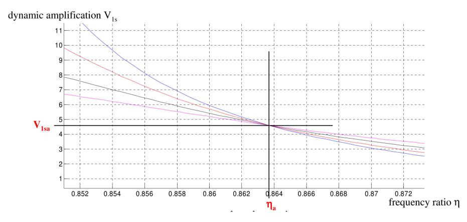
All resonance curves pass through 2 common points  $\eta_a$  and  $\eta_b$ . The frequencies  $\eta_a$  and  $\eta_b$  as well as  $V_{1sa}$  and  $V_{1sb}$  depend on  $\kappa$ and  $\mu$ .
