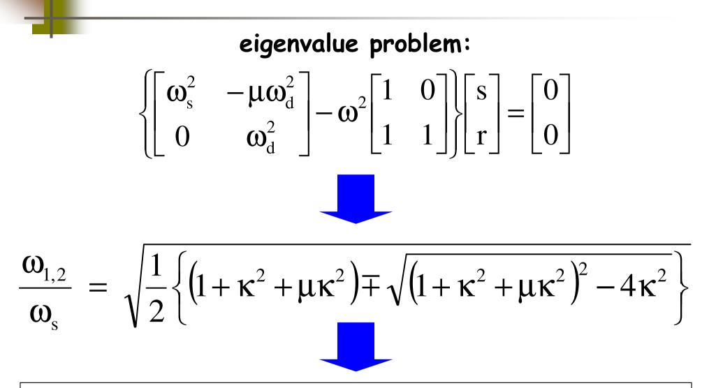
The original single eigenfrequency of the system without TMD is split into two distict eigenfrequencies.
