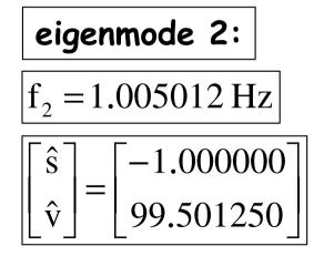
Structure and damper move out of phase!
