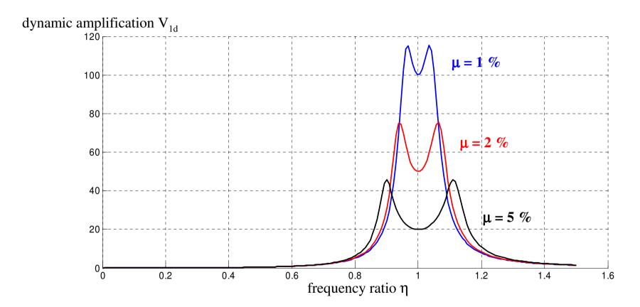
The mass ratio  $\mu$  influences the response of the TMD. A small TMD must produce large amplitudes in order to work.
