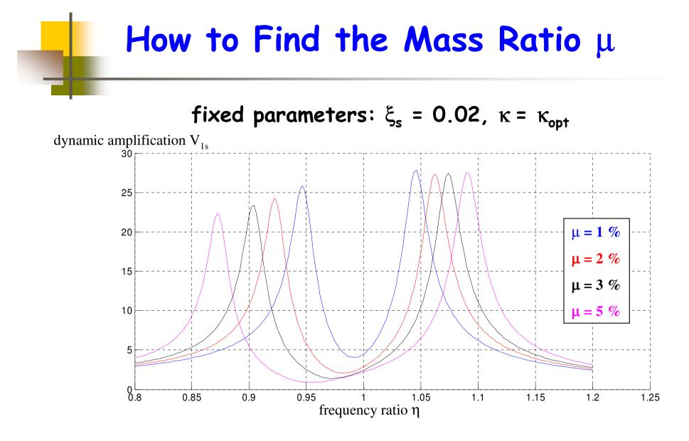
The plateau between the response peaks is widened by a larger  $\mu$  which increases the bandwidth of effectiveness. Common are values of 1 % to 5 % of the *modal* mass for  $\mu$ .
