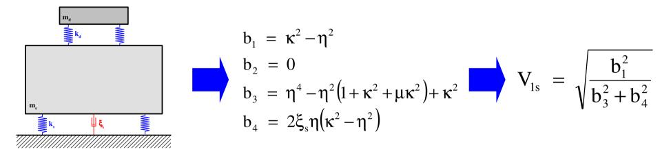
The oscillation of the structure becomes zero if the damper has the same eigenfrequency as the load:  $\omega_d = \Omega$ .
