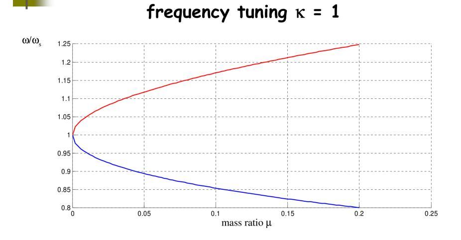
The split of the eigenfrequencies grows more pronounced with increasing mass of the TMD. How does the coupled structure vibrate?
