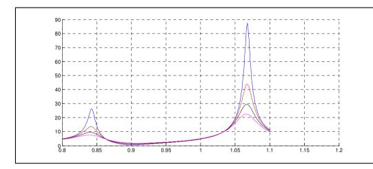
The sensitivity is not symmetric: the amplification is more sensitive with respect to positive rather than negative deviations from  $\eta_{target}$ .
