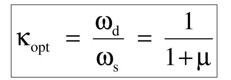
The mass ratio m controls the split of the eigenfrequencies and therefore the width between the two peaks.
